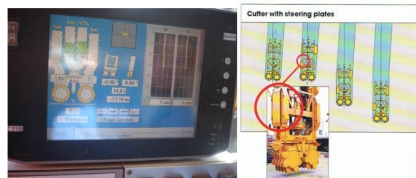
Figures 9a and 9b. Verticality Control System
